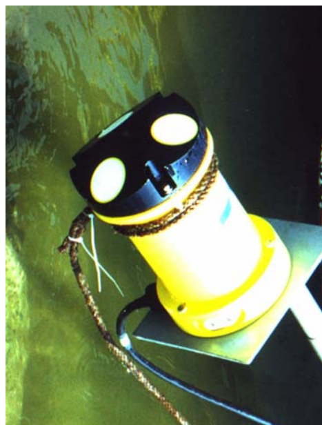
Figure 6.42(b): View on SonTek APD unit
