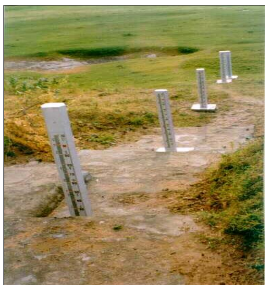
Figure 8.1: Typical Staff Gauge Installation Arrangements
