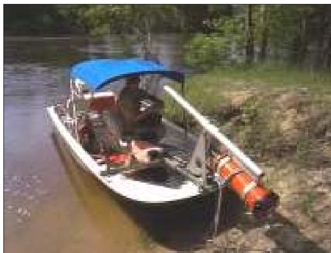
Figure 6.43(b): ADCP and boat
