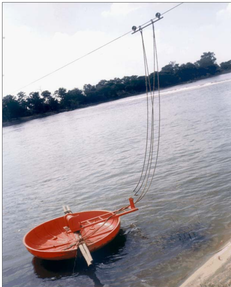
Figure 6.32: Boat gauging - boat cableway system
