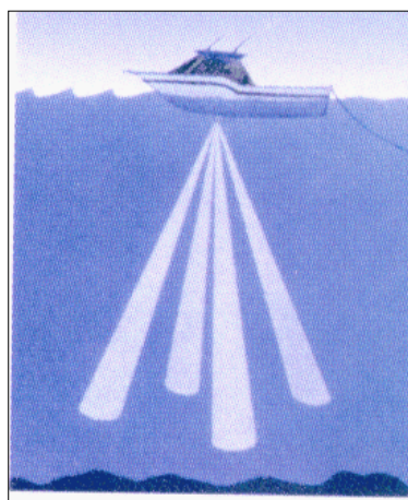
Figure 6.43(a): Acoustic signals for the ADCP
