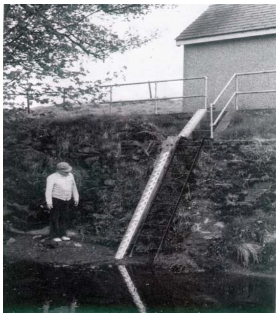
Figure 6.3: Inclined staff gauge
